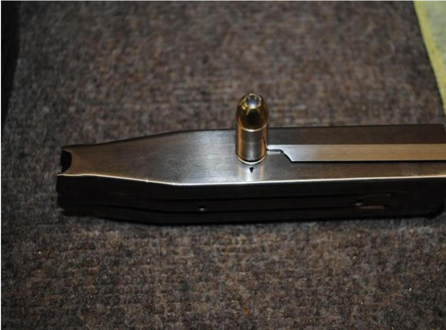
Mark that location with a sharpie and then with a 3/16" drill bit, drill a hole in the tube where the primer will be when the mag is loaded. I use a drill press for this but you can hold the mag in your vise and manually drill it if you don't have one. Keep in mind, the mag tubes are heat treated 410 stainless steel and they are pretty hard.
