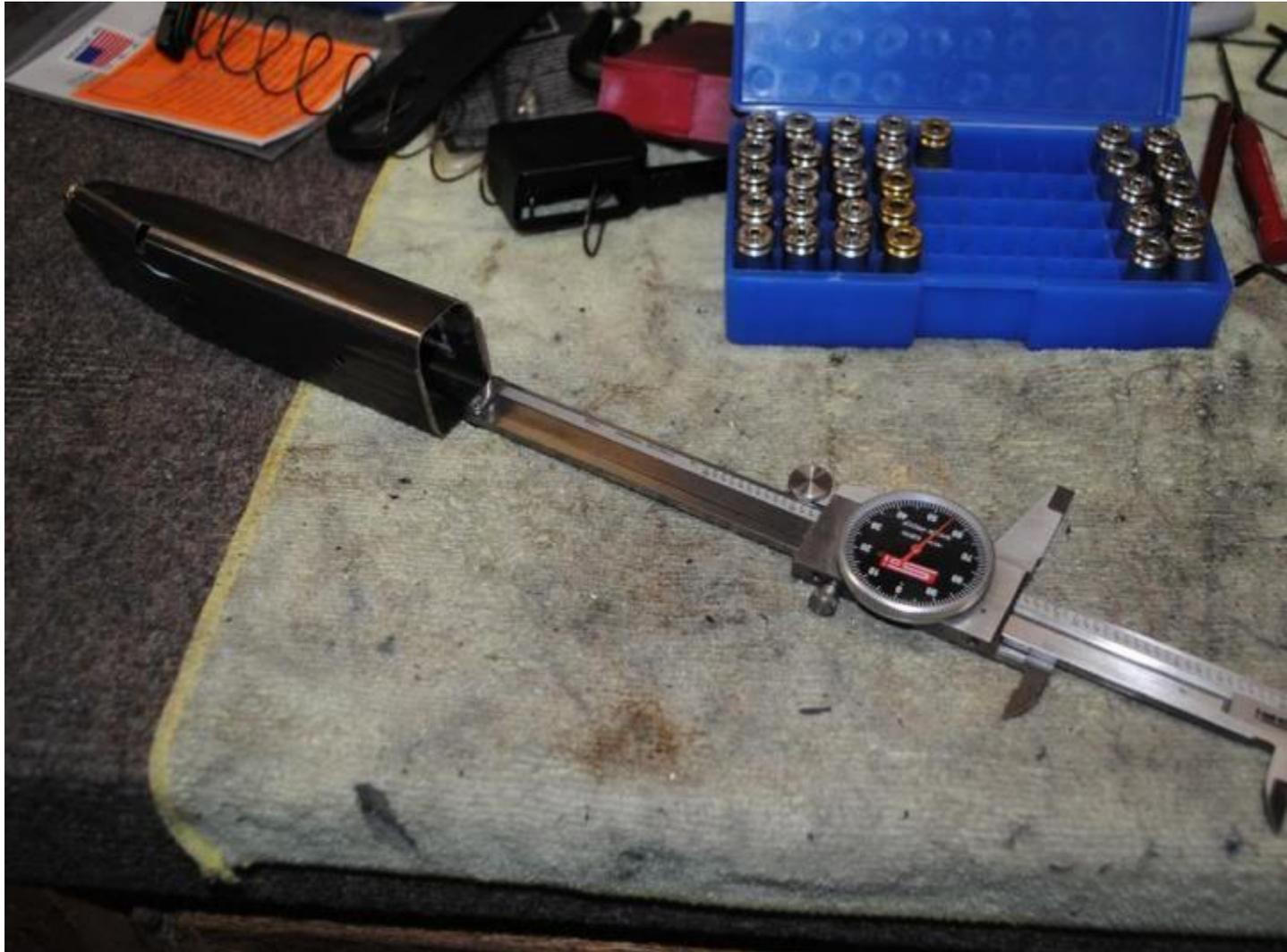
Lock the caliper in place and empty the mag. Now turn your mag front side down on your work bench and lay the drop arm on top of the back of the mag and place a round at the end of the drop arm. The center of that round is where you want your hole.
